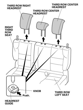
Push the knob and remove the headrests from the third row seats. 3. Install the two third row headrest covers and third row center headrest cover to the three headrests as shown.
