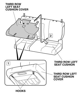
Secure the third row left seat cushion cover to the third row left seat cushion with the two hook-andloop fasteners.
